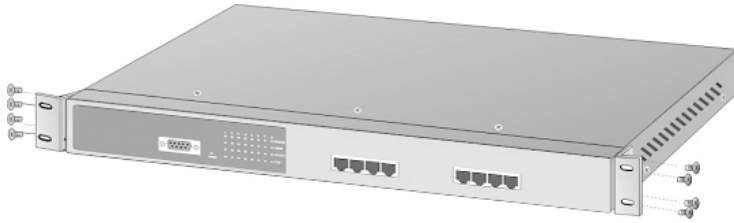
Figure 3-2. Attach mounting brackets with screws
