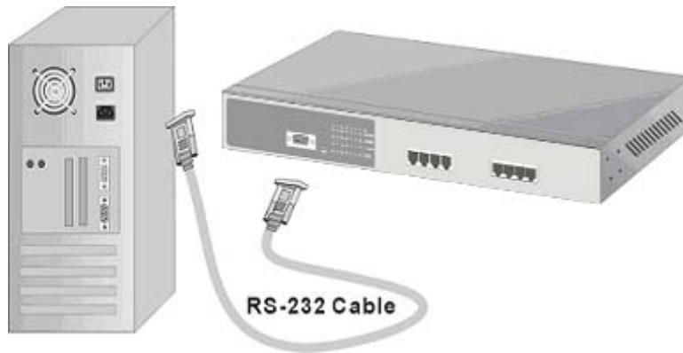
Figure 5-1. Connecting the MIL-S8000G Switch to a terminal via RS-232 cable.
